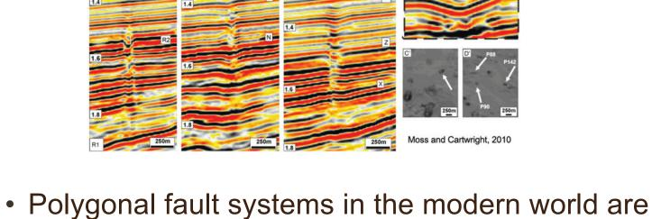
commonly overlain by "pockmarks" on the seafloor (left above), depressions typically a few 100 m across. Seismic lines show concave up reflectors in a sequence
